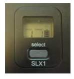
On the front of the transmitter is a small display which shows the state of the batteries. When it shows three bars, they MAY BE okay. Otherwise, you should replace the batteries.
