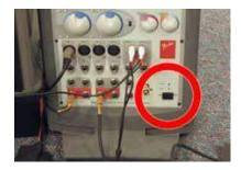
The illustration to the left shows where the power toggle switch is located, at the bottom right of the **Fender** audio controller.
