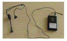
The microphone set consists of the microphone itself, attached to a flexible stem which connects to the wire headgear, then to a cable to the transmitter/battery box and antenna.
