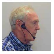
Note in the illustration to the left how the back of the headgear is low on the head, the microphone is on the right side, and the arcs are snug over the ears.
